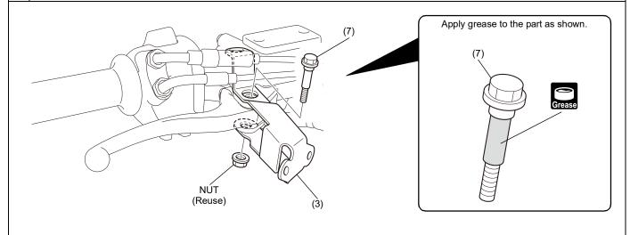
11. Install the parts and tighten the loosely installed parts securely.Tighten the pivot bolt first.
